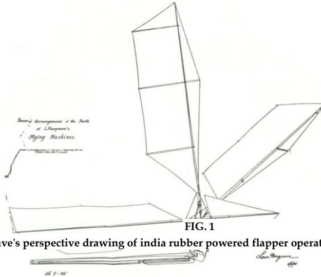
Hargrave's perspective drawing of india rubber powered flapper operated flying machine of 1885
