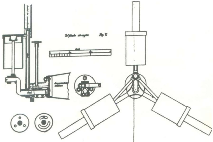
Hargrave's drawing of the three cylinder radial rotary compressed air engine invented 1889
